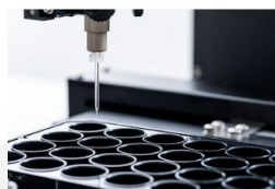
Single-use glass capillary for clone picking
